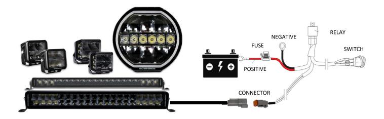
STEP 1: When routing wire harness through any metal surface be sure it is free of any sharp edges and protected using wire sheathing or a grommet.
